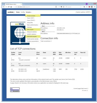
interface. This makes it very portable and accessible. The only requirement is a browser, no drivers are needed to support access on any operating system. The user interface can be scaled depending on resources and requirements from traditional basic HTML to sophisticated modern interfaces using Javascript, Ajax, SSE, Websockets and more.
