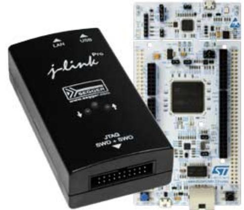
The upgrade turns a board's ST-LINK interface into a fully functional J-Link, which can then be employed to debug the board's application processor. By upgrading to the J-Link firmware, developers will subsequently be able to set an unlimited number of breakpoints in Flash memory and debug their applications considerably faster - resulting in better use of engineering resources and shortened time to market.
