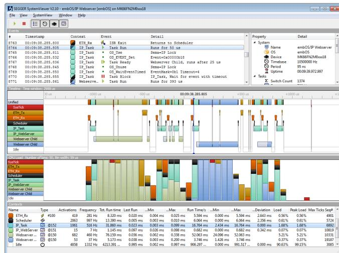
Using SEGGER's J-Link debug probe with SystemView gives the ultimate advantage of streaming data transfer: Unlimited recording capacity and analysis in real-time, working as a live software oscilloscope. This is a great means to gain a deep understanding of the runtime behavior of an application. Real-time analysis is particularly beneficial when developing and working in complex systems with multiple threads and events, and also in bare-metal systems without any RTOS.
