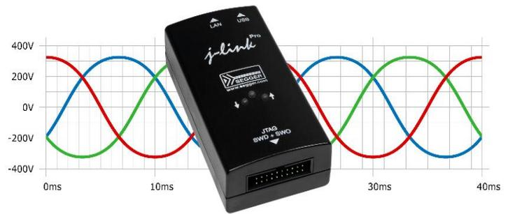
J-Scope is based on the newly introduced J-Link HSS (High Speed Sampling) feature, which makes it possible to continuously sample variables at extremely high speeds without affecting the real-time nature of the embedded device. Using the standard debug interface, it does not require any extra resources on the target such as memory, CPU time or extra pins.
