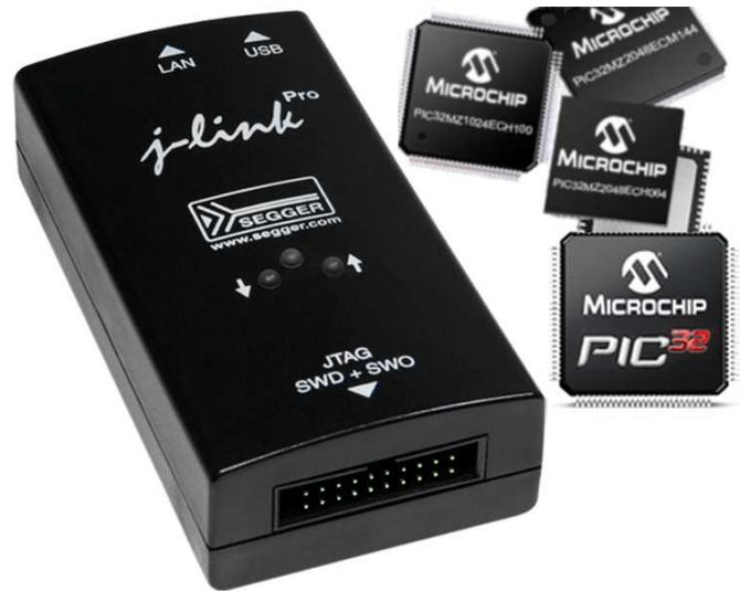
The J-Link is known for having the highest download speed into RAM and flash memory on all supported targets. This is not different when it comes to debugging PIC32 devices. In addition, the J-Link allows setting an unlimited number of breakpoints in flash memory.
