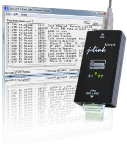
time via the CPU, its main use is to handle terminal output in real-time with very low intrusion. This permits most programs to perform debug outputs via terminal without losing their real-time behavior. More information about J-Link SWOViewer: <a href="http://www.segger.com/j-link-swo-viewer.html">http://www.segger.com/j-link-swo-viewer.html</a>
