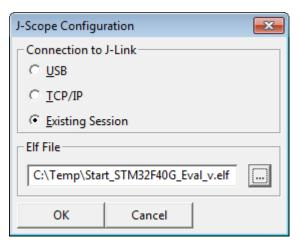
J-Scope can be used alongside other applications, e.g. a debugger, which are connected to J-Link and share the connection to the J-Link. If J-Scope is used in this mode select "Existing Session" as connection type. All Target options will be disabled, as they are already determined by the running session.
