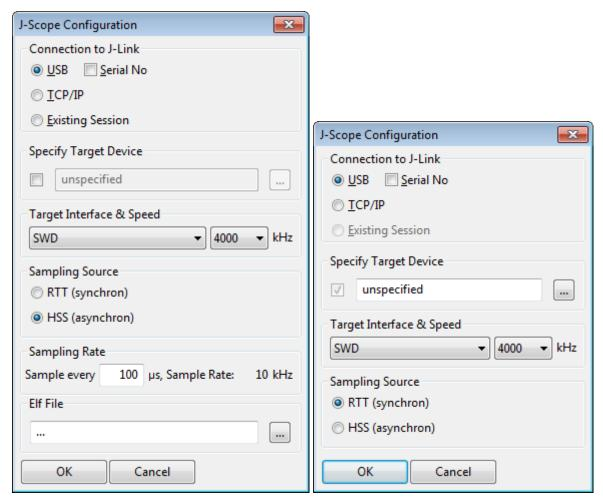
If J-Scope is used in standalone mode, opening a dedicated connection to J-Link, choose "USB" or "TCP/IP" as connection type and optionally enter the serial number or the IP of the J-Link to connect to a specific J-Link.
