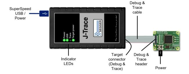
J-Trace ships with a 20-pin, 0.05"-pitch ribbon cable. In rare cases, depending on the target board, you might need a separate trace adapter.
