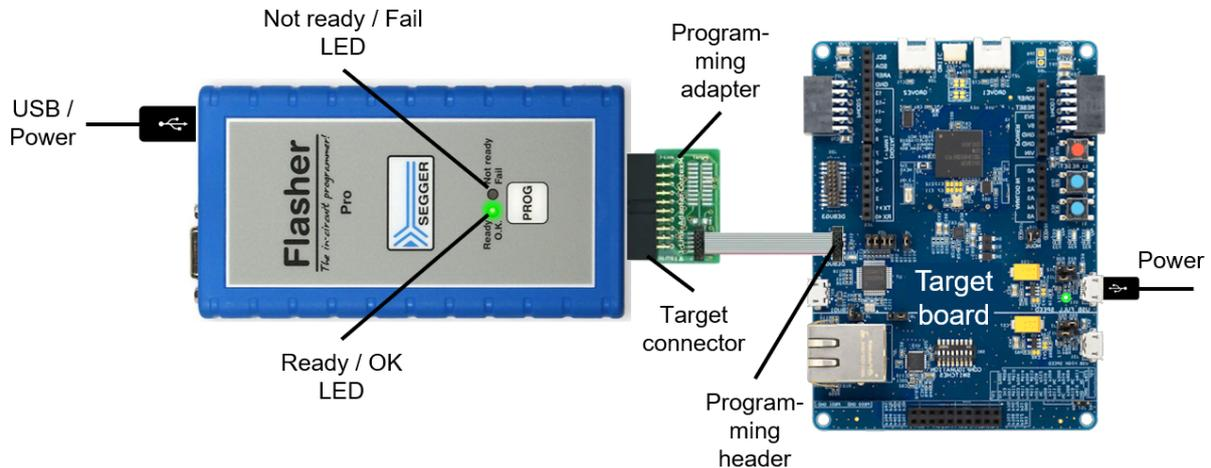
Connect the programming adapter (or the 20-pin ribbon cable, if possible) to the Flasher target connector as well as the programming header on the target board as shown in the image above. Watch out for the correct orientation. The colored wire of the ribbon cable needs to connect to pin 1 of the programming header. Also make sure the connector covers both rows of the programming header.
