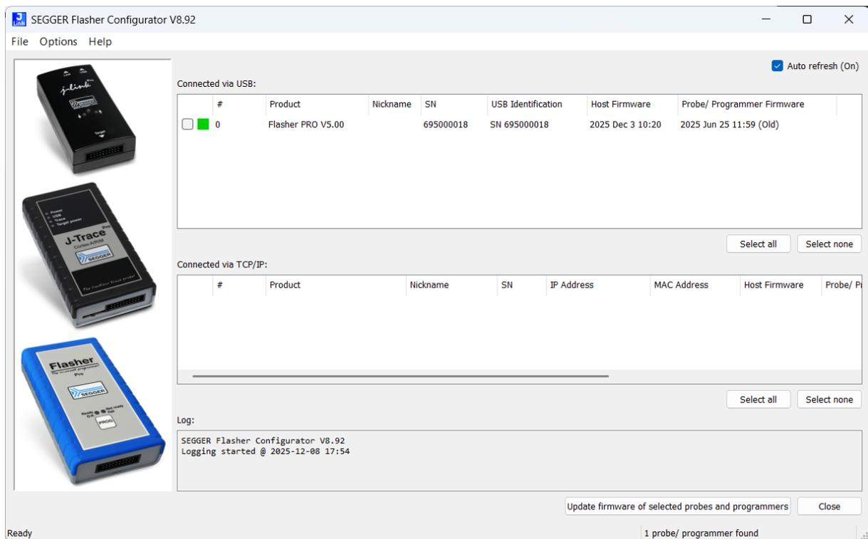
If Flasher Configurator detects that a firmware update is available for the Flasher, it will indicate this by marking the programmer firmware version as "Old" (as shown in the screenshot above).
