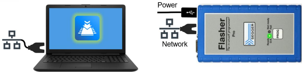
The Flasher Pro will obtain an IP address via DHCP, after which the green Ready / OK LED will slightly flicker once a second. You can check the IP address assigned to the Flasher Pro using the Flasher Configurator utility (also see further below).
