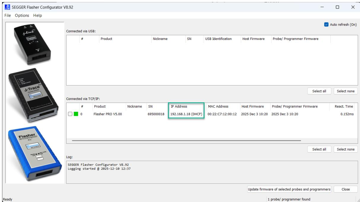
Close down Flasher Configurator after you're done with it, or at least turn off the auto-refresh feature. Since Flasher Configurator constantly looks for SEGGER probes and programmers connected via USB or Ethernet if the auto-refresh is enabled, it might interfere with the operation of these probes / programmers at the same time.
