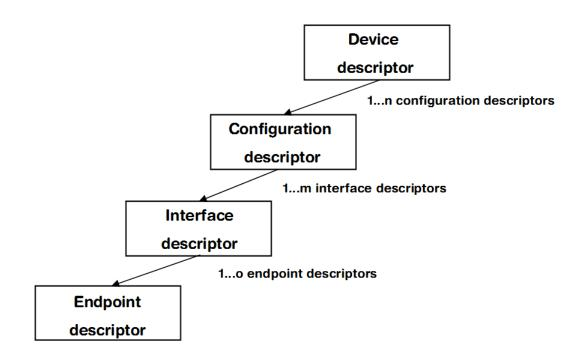
As can be seen, the descriptors form a tree. The root is the device descriptor with n configuration descriptors as children, each of which has m interface descriptors which in turn have o endpoint descriptors each.
