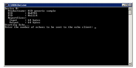
4. Enter the number of reports that should be transmitted when the device is connected. Every dot in the terminal window indicates a transmission.
