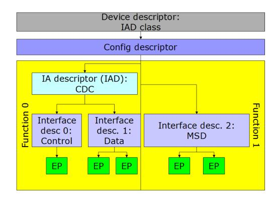
Since IAD is an extension to the original USB specification, it is not supported by all hosts, especially older host software. If IAD is not supported, the device may not be enumerated correctly.
