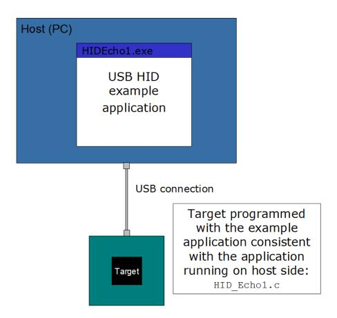
To use this application, include the source code file <code>USB\_HID\_Echol.c</code> into your project and compile and download it into your target. Run <code>HIDEchol.exe</code> after the target is connected to the host and the enumeration process has been completed. The PC application is supplied as executable in the <code>Windows\USB\HID\SampleApp\Exe</code> directory. The source code of the
