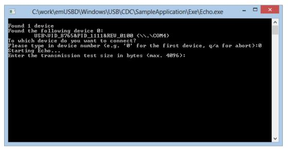
Now enter the number of repetitions the application shall send and receive to or from device and confirm with [Enter]..
