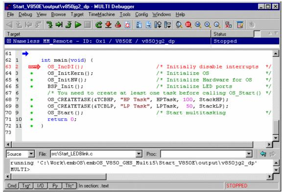
Before you step into OS\_Start(), you should set breakpoints into the two tasks.
