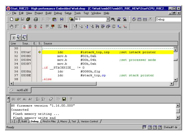
The Debugger will load the file and show the startup code:
