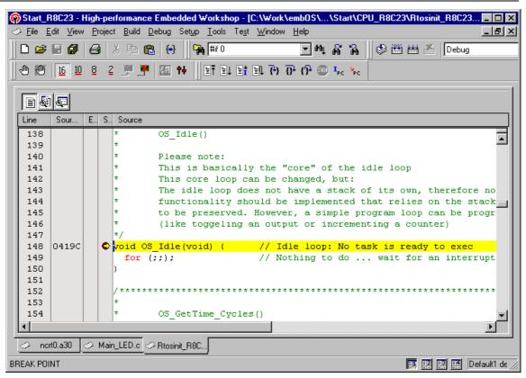
If you set a breakpoint in one or both of our tasks, you will see that they continue execution after the given delay. You may open the watch window to display the *embOS* time variable OS\_Time, which shows how much time has expired in the target system.
