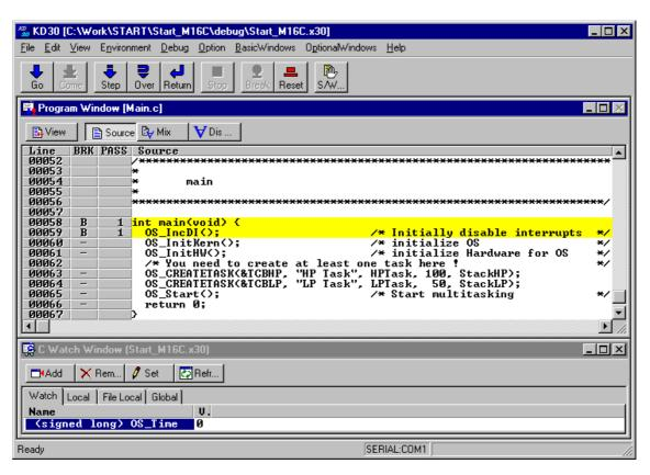
OS\_IncDI() initially disables interrupts and informs *embOS* that interrupts should not be re-enabled during *embOS* function calls.
