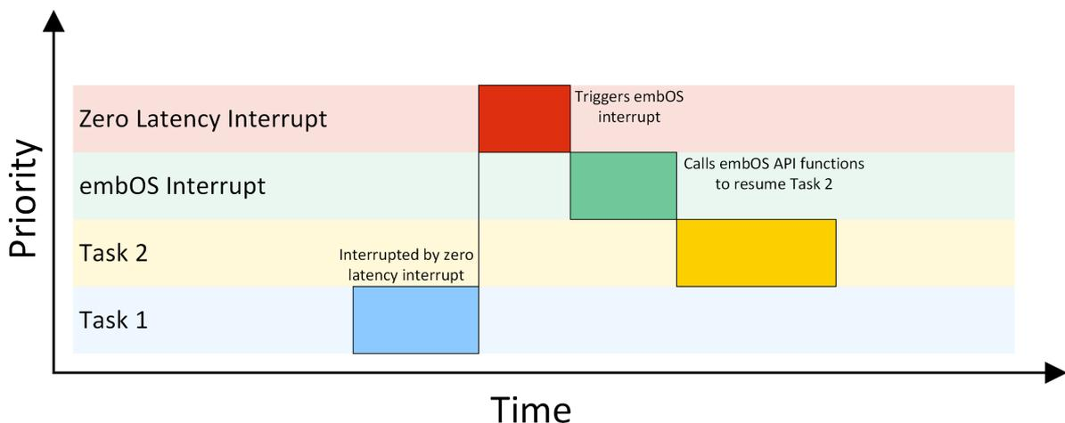
The task 1 is interrupted by a high priority interrupt. This high priority interrupt is not allowed to call an embOS API function directly. Therefore the high priority interrupt triggers a low priority interrupt, which is allowed to call embOS API functions. The low priority interrupt calls an embOS API function to resume task 2.
