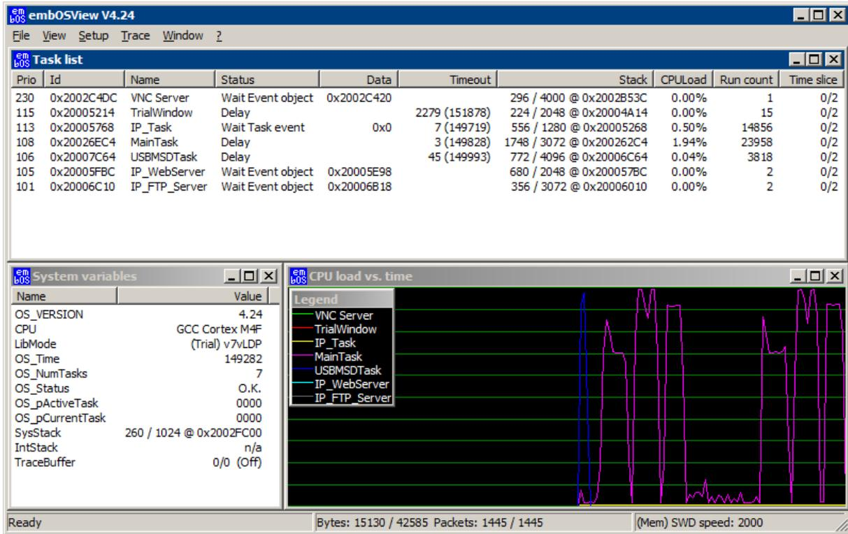
Most often, a serial interface (UART) is used for the communication with the target hardware. Alternative communication channels include Ethernet, memory read/write for Cortex-M and RX CPUs, and DCC for ARM7/9 and Cortex-A CPUs. The hardware dependent routines and defines available for communication with embOSView are implemented inside the source file RTOSInit.c. Details on how to modify this file are also included in *How to change settings* on page 458.
