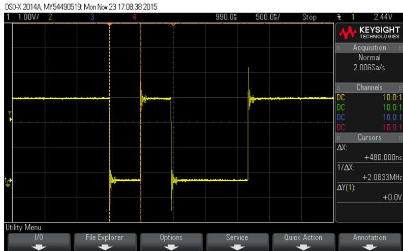
$t_{CD}$  is measured as 12000ns.
