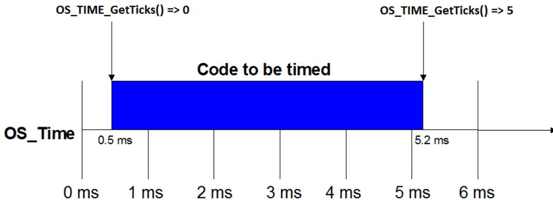
For many applications, low-resolution measurement is sufficient for most of all cases. In those cases, its ease of use as well as its faster computation time are clear benefits when compared to high-resolution measurement. Still, high-resolution measurement may be necessary when highly accurate measurements are mandatory.
