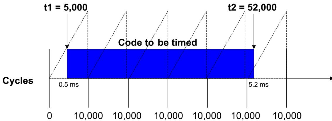
The call to `OS_TIME_StartMeasurement()` calculates the starting value at 5,000 cycles, while the call to `OS_TIME_StopMeasurement()` calculates the ending value at 52,000 cycles (both values are kept track of internally). The measured execution time of the code in this example would therefore be  $(52,000 \text{ cycles} - 5,000 \text{ cycles}) = 47,000 \text{ cycles}$ , which equals 4.7 msec.
