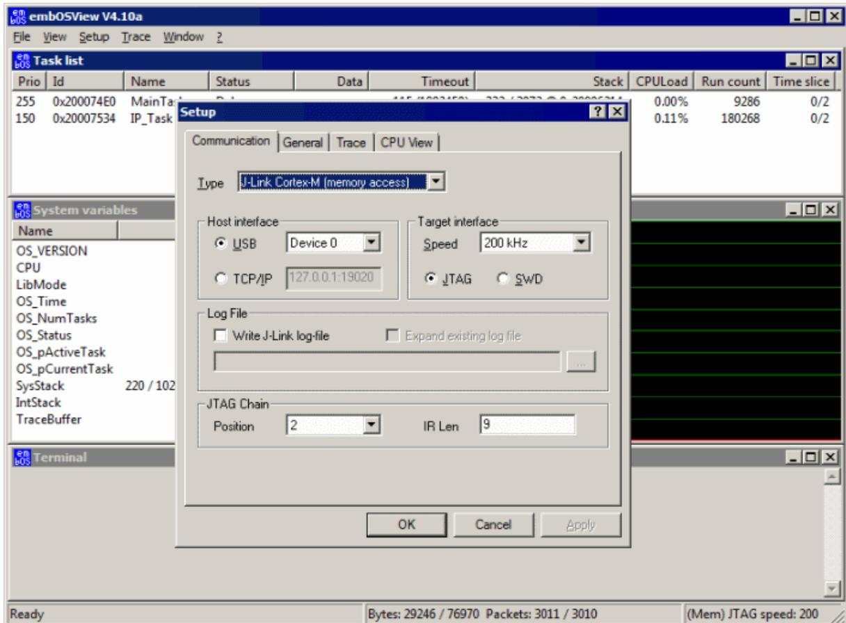
In the Communication tab, choose J-Link Cortex-M (memory access), J-Link RX (memory access) or J-Link ARM7/9/11 (DCC) in the Type selection listbox.
