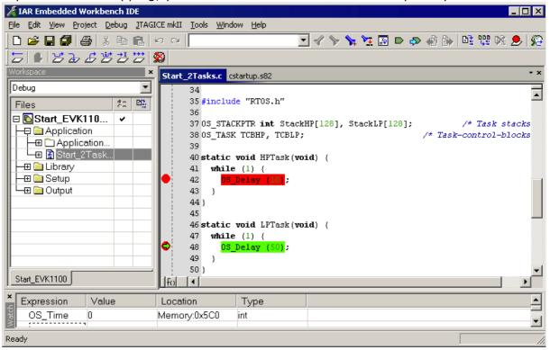
Continuing to step through the program, there is no other task ready for execution. **embOS** will therefore start the idle-loop, which is an endless loop which is always executed if there is nothing else to do (no task is ready, no interrupt routine or timer executing).
