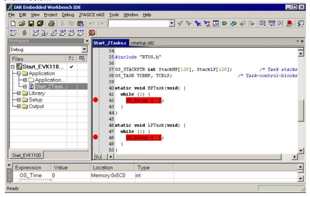
As <code>OS\_Start()</code> is part of the <code>embOS</code> library, you can step through it in disassembly mode only. You may press <code>GO</code>, step over <code>OS\_Start()</code>, or step into <code>OS\_Start()</code> in disassembly mode until you reach the highest priority task.
