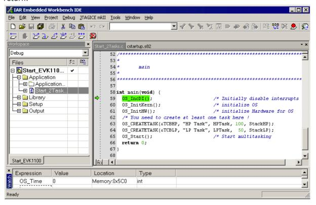
Before you step into  $OS\_Start()$ , you should set two break points in the two tasks as shown below.
