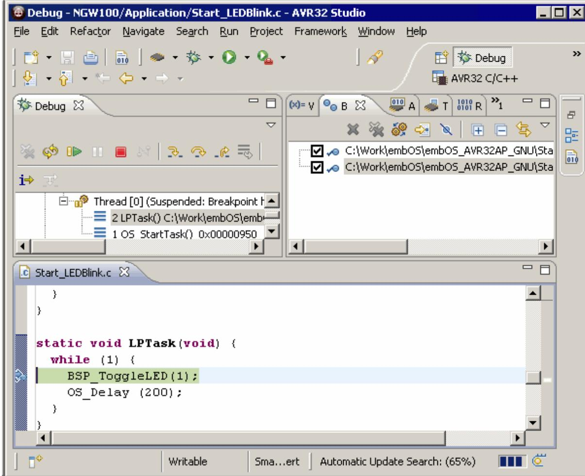
Continuing to step through the program, there is no other task ready for execution. **embOS** will therefore start the idle-loop, which is an endless loop which is always executed if there is nothing else to do (no task is ready, no interrupt routine or timer executing).
