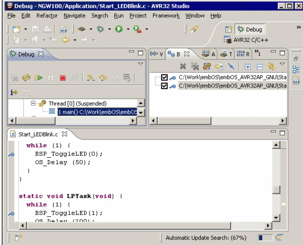
As `OS_Start()` is part of the **embOS** library, you can step through it in disassembly mode only. You may press **GO**, step over `OS_Start()`, or step into `OS_Start()` in disassembly mode until you reach the highest priority task.
