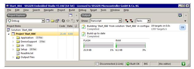
For additional information, you should open the ReadMe.txt file that is part of every BSP. It describes the different configurations of the project and, if required, gives additional information about specific hardware settings of the supported evaluation board(s).
