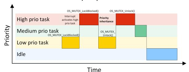
With priority inheritance, the low priority task inherits the priority of the waiting high priority task as long as it holds the mutex. The lower priority task is activated instead of the medium priority task when the high priority task tries to claim the mutex.
