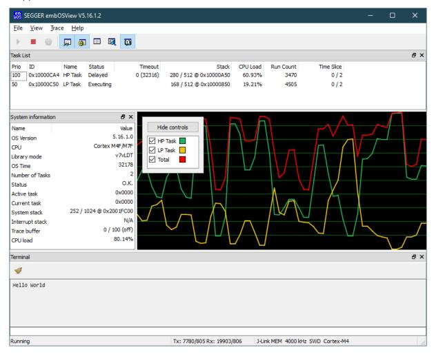
Most often, a serial interface (UART) is used for the communication with the target hardware. Alternative communication channels include Ethernet, memory read/write for Cortex-M and RX CPUs, as well as DCC for ARM7/9 and Cortex-A/R CPUs. The hardware dependent routines and defines available for communication with embOSView are implemented in the source file RTOSInit.c. Details on how to modify this file are also given in chapter Setup target for communication on page 500.
