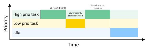
If tasks in a pure cooperative multi-tasking system do not cooperate, the system "hangs". This means that other tasks have no chance of being executed by the CPU while the first task is being carried out. Even if an ISR makes a higher-priority task ready to run, the interrupted task will be resumed and completes before the task switch is made.
