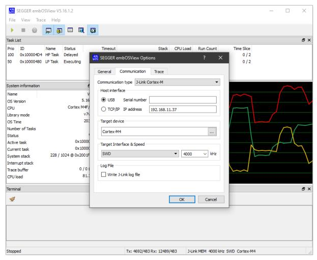
In the Communication tab, choose "J-Link Cortex-M (memory access)", "J-Link RX (memory access)" or "J-Link ARM7/9/11 (DCC)" in the  $_{\mathrm{Type}}$  selection list box.
