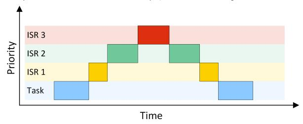
For applications requiring short interrupt latency, you may re-enable interrupts inside an ISR by using  $OS_INT_EnterNestable()$  and  $OS_INT_LeaveNestable()$  within the interrupt handler.
