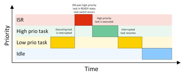
Preemptive multitasking may be switched off in sections of a program where task switches are prohibited, known as critical regions. embOS itself will also temporarily disable preemptive task switches during critical operations, which might be performed during the execution of some embOS API functions.
