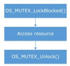
A mutex contains a counter that keeps track of how many times the mutex has been claimed by calling  $os_{tock}()$  or  $os_{tock}()$  or  $os_{tock}()$  by a particular task. It is released when that counter reaches zero, which means the  $os_{tock}()$  routine must be called exactly the same number of times as  $os_{tock}()$  or  $os_{tock}()$  or  $os_{tock}()$ . If it is not, the mutex remains blocked for other tasks.
