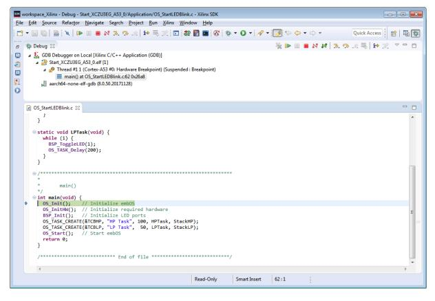
Before you step into <code>OS\_Start()</code>, you should set two breakpoints in the two tasks as shown below.
