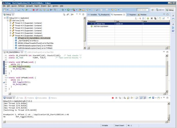
Continuing to step through the program, the  $\mathtt{LPTask}()$  will switch on LED1 and then run into its delay.
