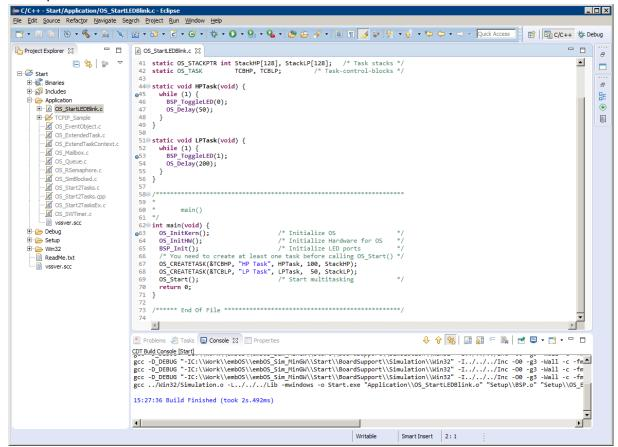
Step over  $os\_start()$ , or step into  $os\_start()$  in disassembly mode until you reach the highest priority task. If you continue stepping, the first LED of your device will be switched on, the HPTask() will run into its delay and therefore, embOS will start the task with lower priority.
