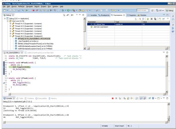
Please note, that delays seem to be longer than expected. When the debugger stops at a breakpoint, it takes some time until the screen is updated and the  $OS_Global.Time$  variable is examined. Therefore  $OS_Global.Time$  may show larger values than expected. After the delay of HPTask() expired, the simulated device shows both LEDs lit as can be seen in the following screenshot:
