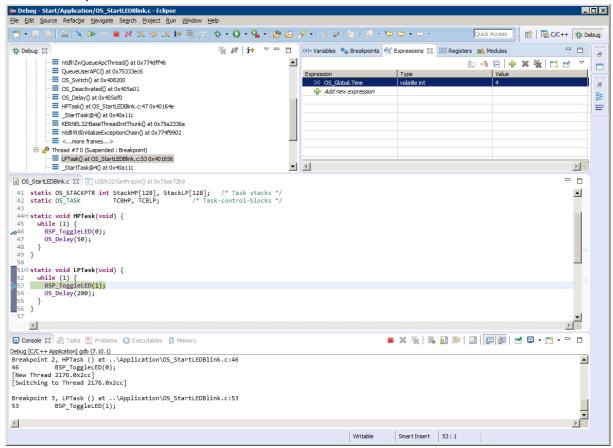
As there is no other task ready for execution when  $\mathtt{LPTask}()$  runs into its delay, embOS will suspend  $\mathtt{LPTask}()$  and switch to the idle process, which is always executed if there is nothing else to do (no task is ready, no interrupt routine or timer executing).
