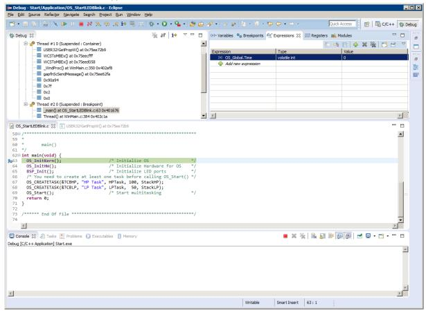
The embOS simulation environment is set up and displays a simulated device which is shown before the debugger stops at the breakpoint at main().
