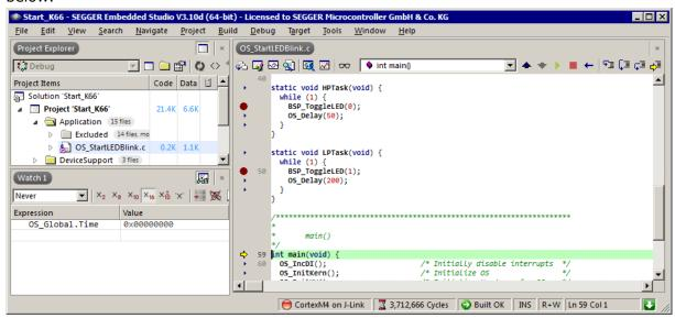
As <code>OS\_Start()</code> is part of the embOS library, you can step through it in disassembly mode only.
