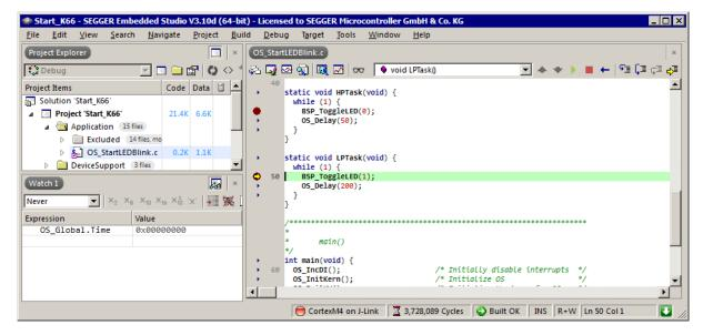
Continue to step through the program, there is no other task ready for execution. embOS will therefore start the idle-loop, which is an endless loop always executed if there is nothing else to do (no task is ready, no interrupt routine or timer executing).
