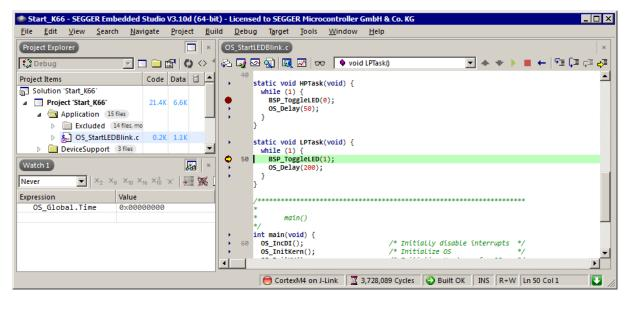
Continue to step through the program, there is no other task ready for execution. embOS will therefore start the idle-loop, which is an endless loop always executed if there is nothing else to do (no task is ready, no interrupt routine or timer executing).
