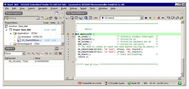
Before you step into <code>OS\_Start()</code>, you should set two breakpoints in the two tasks as shown below.
