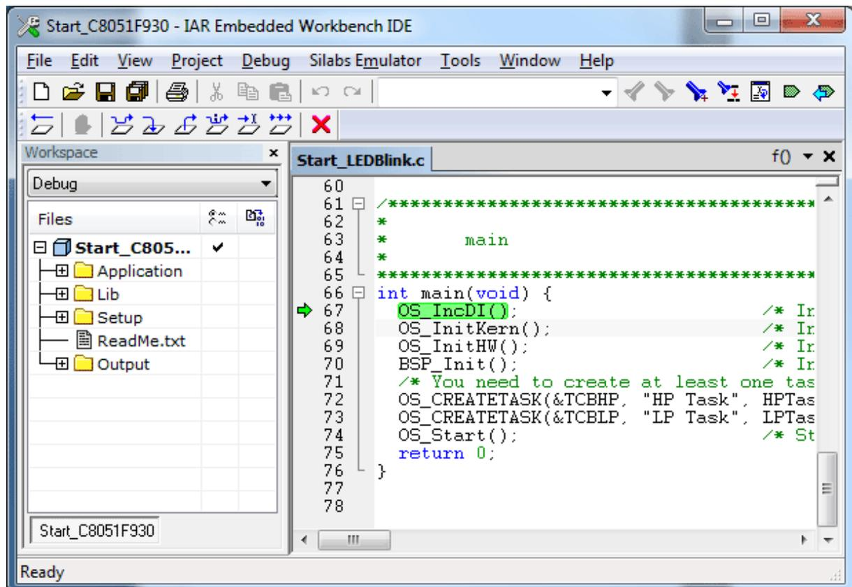
Before you step into `OS_Start()`, you should set two breakpoints in the two tasks as shown below.
