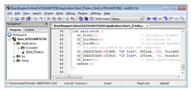
Before you step into  $OS\_Start()$ , you should set two breakpoints in the two tasks as shown below.
