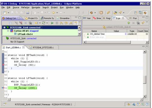
Continue to step through the program, there is no other task ready for execution. embOS will therefore start the idle-loop, which is an endless loop always executed if there is nothing else to do (no task is ready, no interrupt routine or timer executing).
