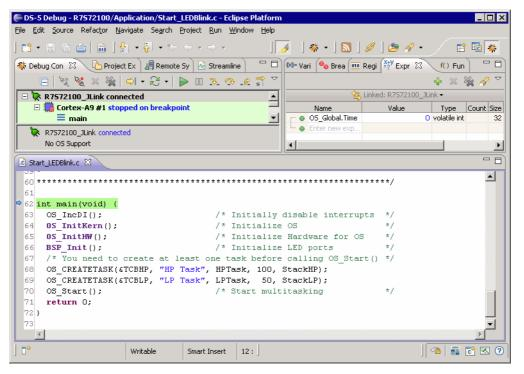
Before you step into  $\texttt{OS\_Start()}$  , you should set two breakpoints in the two tasks as shown below:
