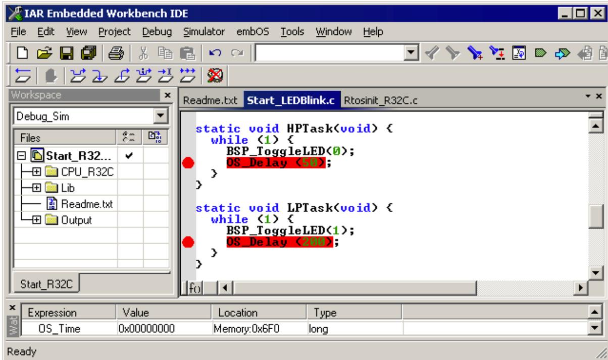
As `OS_Start()` is part of the embOS library, you can step through it in disassembly mode only. Click **GO**, step over `OS_Start()`, or step into `OS_Start()` in disassembly mode until you reach the highest priority task.
