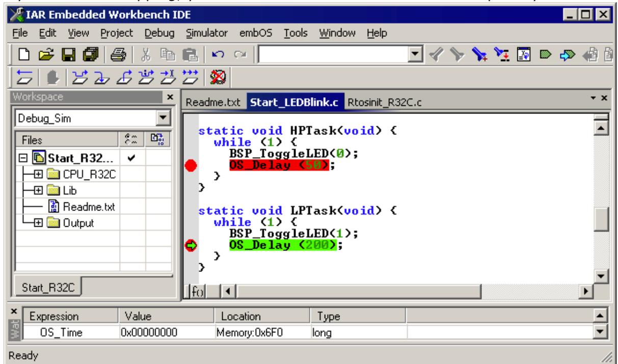
Continue to step through the program, there is no other task ready for execution. embOS will therefore start the idle-loop, which is an endless loop which is always executed if there is nothing else to do (no task is ready, no interrupt routine or timer executing).
