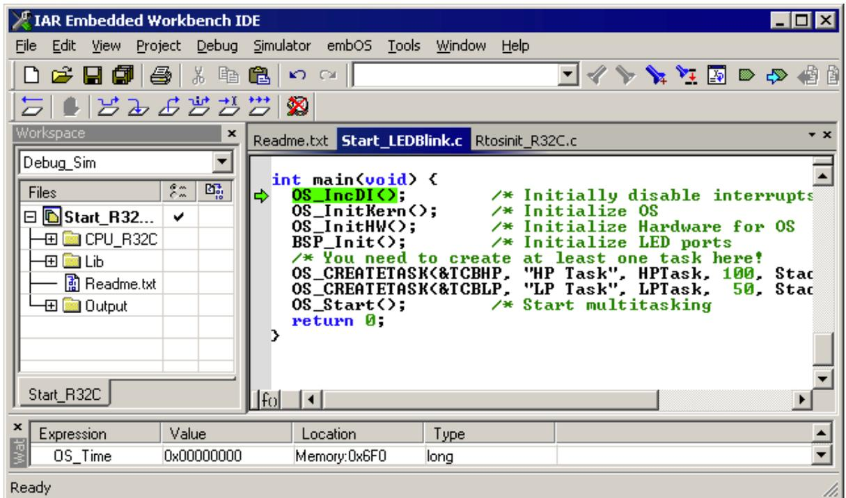
Before you step into `OS_Start()`, you should set two breakpoints in the two tasks as shown below.
