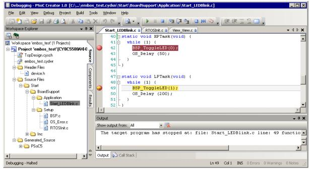
Continue to step through the program, there is no other task ready for execution. embOS will therefore start the idle-loop, which is an endless loop always executed if there is nothing else to do (no task is ready, no interrupt routine or timer executing).
