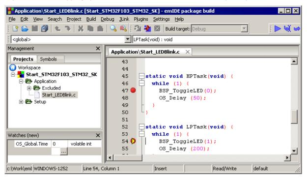
Continue to step through the program, there is no other task ready for execution. embOS will therefore start the idle-loop, which is an endless loop always executed if there is nothing else to do (no task is ready, no interrupt routine or timer executing).
