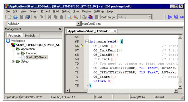
Before you step into <code>OS\_Start()</code>, you should set two breakpoints in the two tasks as shown below.
