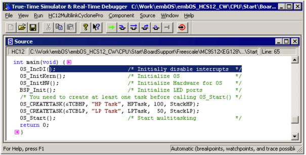
Before you step into  ${\tt OS\_Start()}$  , you should set two breakpoints in the two tasks as shown below.
