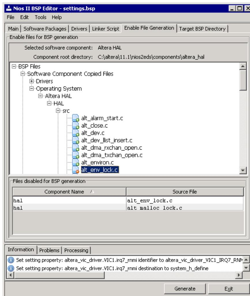
After disabling the two source files from generation, three additional header files which were delivered with embOS have to be disabled from generation. Browse through `Software Component Copied Files -> Operating System -> HAL -> inc -> os`, select the
