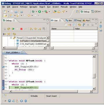
Continue to step through the program, there is no other task ready for execution. embOS will therefore start the idle-loop, which is an endless loop always executed if there is nothing else to do (no task is ready, no interrupt routine or timer executing).
