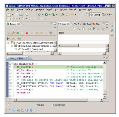
Before you step into <code>OS\_Start()</code>, you should set two breakpoints in the two tasks as shown below.
