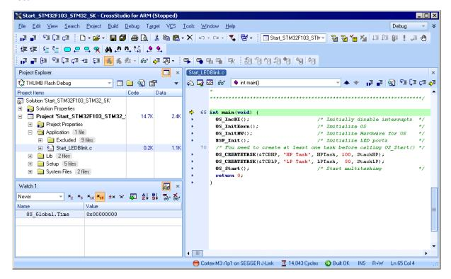
Before you step into <code>OS\_Start()</code>, you should set two breakpoints in the two tasks as shown below.
