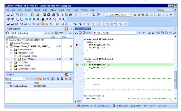
Continue to step through the program, there is no other task ready for execution. embOS will therefore start the idle-loop, which is an endless loop always executed if there is nothing else to do (no task is ready, no interrupt routine or timer executing).
