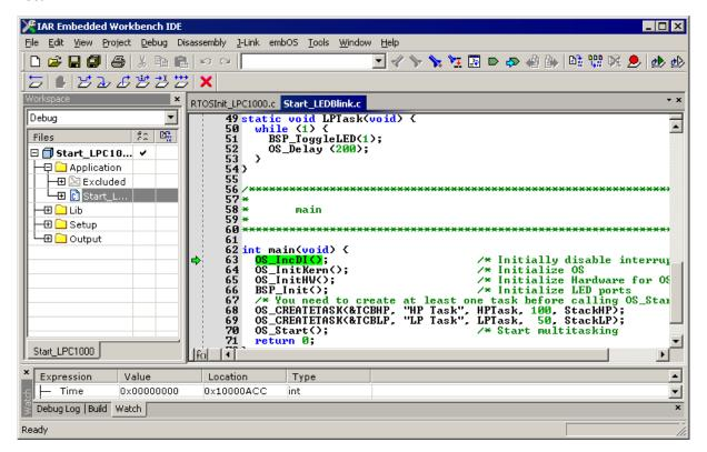
Before you step into <code>OS\_Start()</code>, you should set two breakpoints in the two tasks as shown below.
