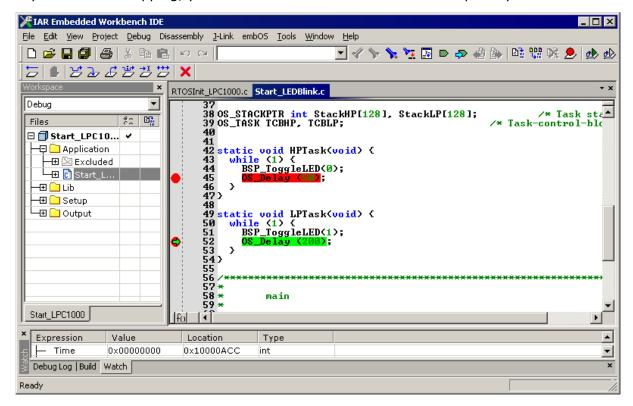
Continue to step through the program, there is no other task ready for execution. embOS will therefore start the idle-loop, which is an endless loop always executed if there is nothing else to do (no task is ready, no interrupt routine or timer executing).
