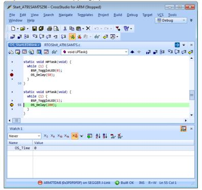
Continue to step through the program, there is no other task ready for execution. embOS will therefore start the idle-loop, which is an endless loop always executed if there is nothing else to do (no task is ready, no interrupt routine or timer executing).
