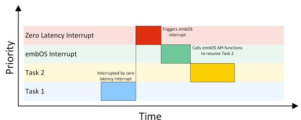
The task 1 is interrupted by a high priority interrupt. This zero latency interrupt is not allowed to call an embOS API function directly. Therefore the zero latency interrupt triggers an embOS interrupt, which is allowed to call embOS API functions. The embOS interrupt calls an embOS API function to resume task 2. How the embOS interrupt gets triggered is device specific and cannot be explained here in general. But with most devices and interrupt
