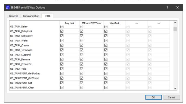
To enable or disable a filter, simply check or uncheck the corresponding checkboxes. For any of these five filters, individual API functions can be enabled or disabled by checking or unchecking the corresponding checkboxes in the list.
