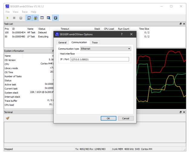
In the Communication tab, choose "Ethernet" in the Type selection list box. In the  ${\tt Host}$  interface box, configure the IP address of your target and the port number  ${\tt 50021}$ .
