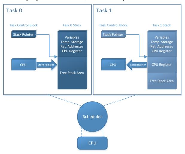
The scheduler deactivates the task to be suspended (Task 0) by saving the processor registers on its stack. It then activates the higher-priority task (Task 1) by loading the stack pointer (SP) and the processor registers from the values stored on Task 1's stack.
