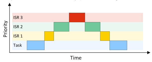
For applications requiring short interrupt latency, you may re-enable interrupts inside an ISR by using <code>OS\_INT\_EnterNestable()</code> and <code>OS\_INT\_LeaveNestable()</code> within the interrupt handler.
