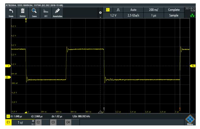
$t_{\text{CD}}$  is measured as 1020ns.
