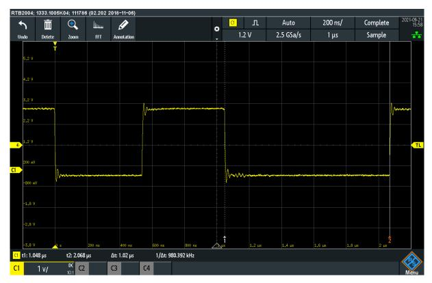
$t_{\text{CD}}$  is measured as 1020ns.
