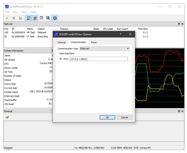
In the Communication tab, choose "Ethernet" in the Type selection list box. In the Host interface box, configure the IP address of your target and the port number 50021.
