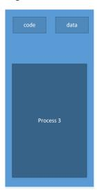
Threads are tasks that share the same memory layout, hence any two threads can access the same memory locations. If virtual memory is used, the same virtual to physical translation and access rights are used.
