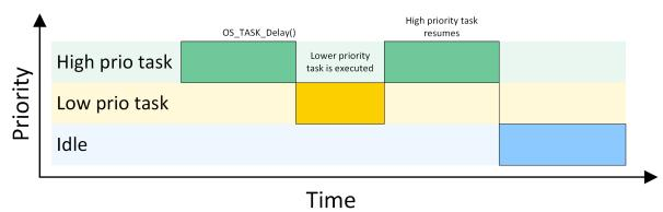
If tasks in a pure cooperative multi-tasking system do not cooperate, the system "hangs". This means that other tasks have no chance of being executed by the CPU while the first task is being carried out. Even if an ISR makes a higher-priority task ready to run, the interrupted task will be resumed and completes before the task switch is made.
