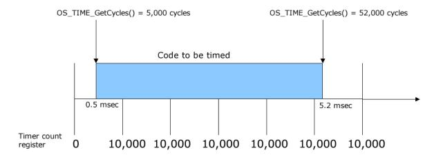
The first call to  $OS_{TIME\_Get\_Cycles()}$  returns the starting value at 5,000 cycles, while the second call to  $OS_{TIME\_Get\_Cycles()}$  returns the ending value at 52,000 cycles. The measured execution time of the code in this example would therefore be (52,000 cycles - 5,000 cycles) = 47,000 cycles, which exactly equals 4.7 millisecond.
