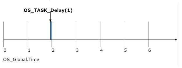
The actual timeout depends on when the API function is called in relation to the next timer interrupt. A timeout of 1 could cause the API function to almost return immediately.
