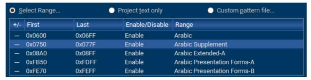
Please keep in mind that for drawing Arabic text the representation forms are very important. Without those representation forms emWin is not able to draw Arabic text. To create the font file for the AppWizard setup the above ranges with 'Default codepoint range...' and then create a new font file with same presets as we used for the first file.
