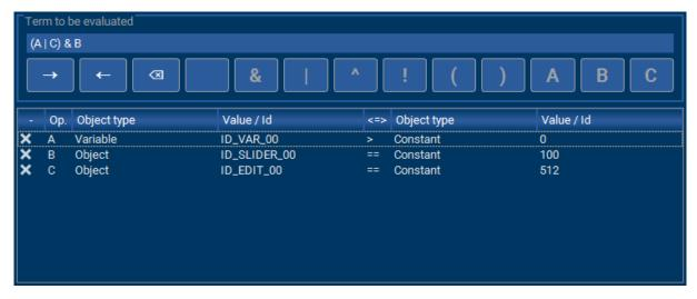
The interface allows the user to enter the term using the buttons or manually enter it via the keyboard. For each operand, an individual button is added.
