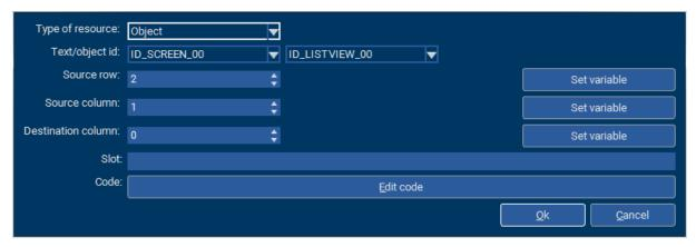
The fields 'Source row' and 'Source column' are not used in any case. If the source is an object with only one field, such as an EDIT or a TEXT object, both specifications are ignored. If the source is a LISTBOX or a DROPDOWN object, only 'Source row' is used. Only with a LISTVIEW object both specifications are used. The same applies to the target object. The 'Destination column' field is only needed if the target object is a LISTVIEW object.
