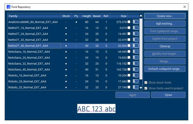
The table shows whether the font is a stock font and/or is used in the project. It also shows how often fonts are referenced in any objects and the height of the font. By ticking the checkbox next to the SD card, the font can be marked as an external resource.
