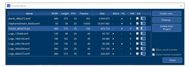
It is important to know that the movie support of AppWizard requires an external tool to convert movies to an emWin compatible format. That tool is FFmpeg which is free available under www.ffmpeg.org. If this tool is not yet set up, the 'Create new...' button is not yet visible.
