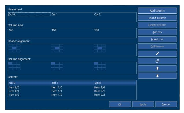
This dialog is used to edit existing content and/or to create new content. Lists consist of simple text arrays. Tables consist of several columns. For each column the width and the alignment can be defined as well as the content of the header.
