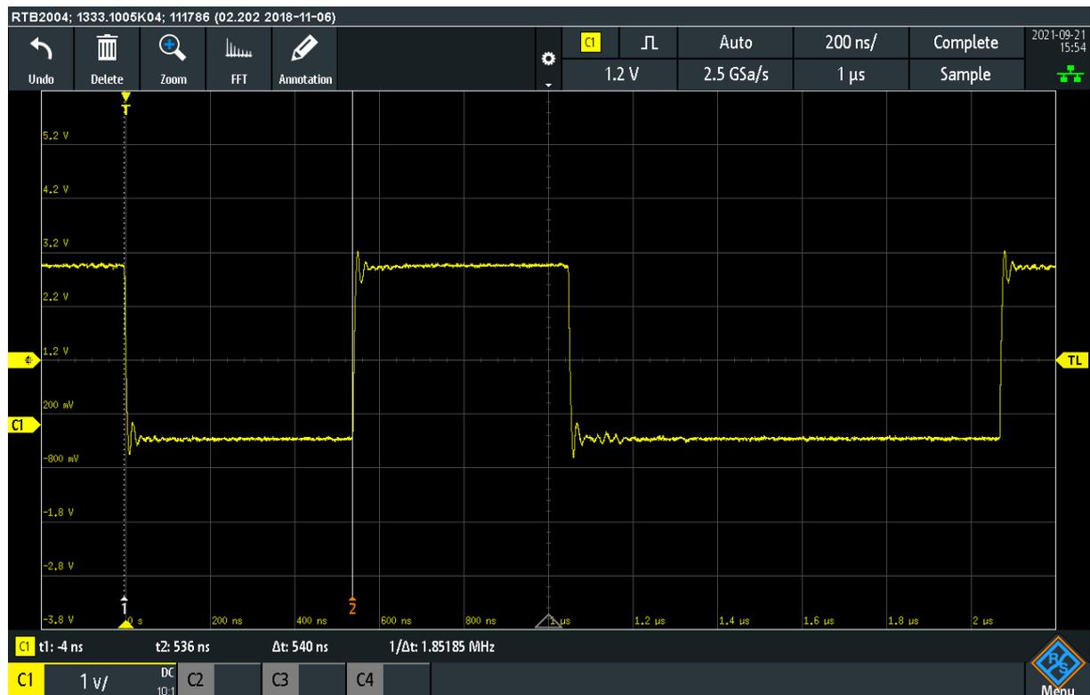
$t_{AB}$  is measured as 540ns.
