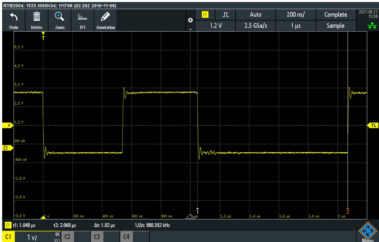
$t_{CD}$  is measured as 1020ns.
