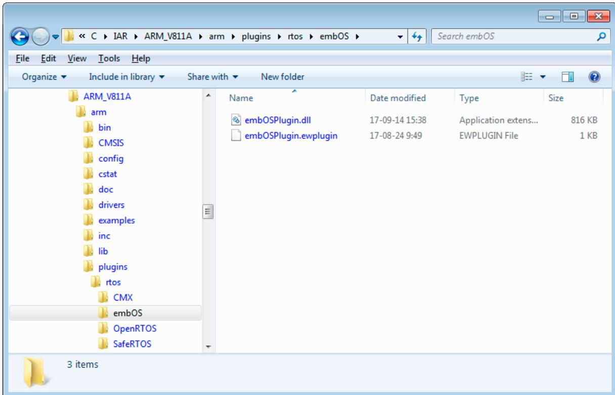
If appropriate folders do not yet exist with your installation, you should create a directory called `embOS` within the CPU specific folder `plugin\rtos\`, and subsequently copy the files from the embOS C-Spy plug-in package into that folder. Note that IAR Embedded Workbench must not be running during the update process.
