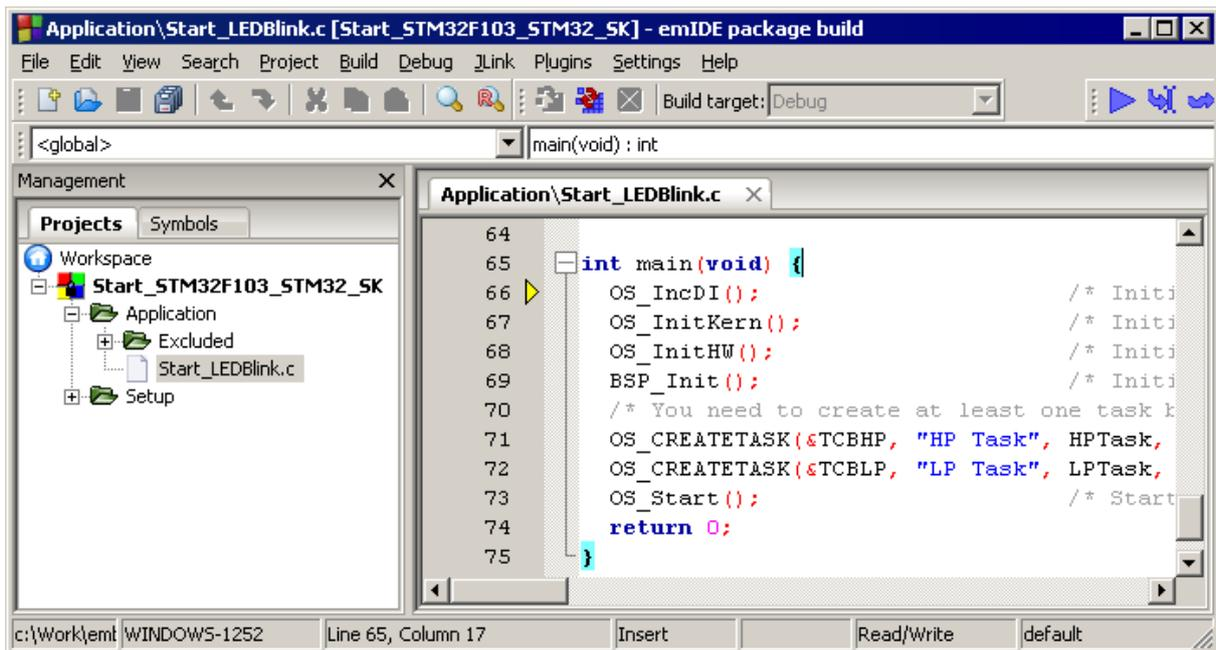
Before you step into `OS_Start()`, you should set two breakpoints in the two tasks as shown below.
