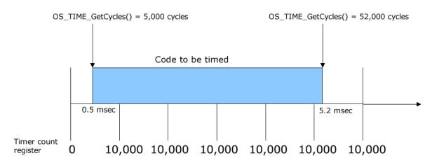
The first call to  $OS_TIME_Get_Cycles()$  returns the starting value at 5,000 cycles, while the second call to  $OS_TIME_Get_Cycles()$  returns the ending value at 52,000 cycles. The measured execution time of the code in this example would therefore be (52,000 cycles - 5,000 cycles) = 47,000 cycles, which exactly equals 4.7 millisecond.
