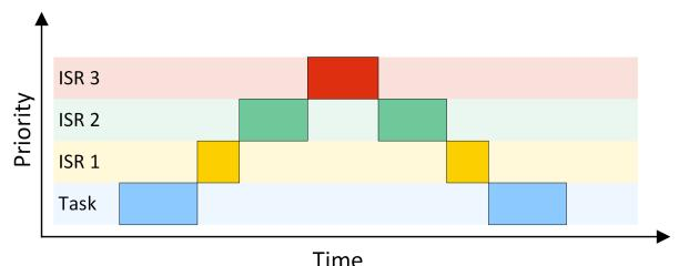
For applications requiring short interrupt latency, you may re-enable interrupts inside an ISR by using <code>OS\_INT\_EnterNestable()</code> and <code>OS\_INT\_LeaveNestable()</code> within the interrupt handler.
