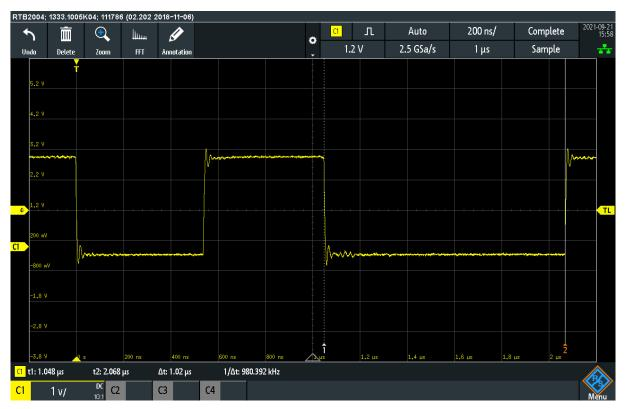
$t_{CD}$  is measured as 1020ns. The number of cycles calculates as follows: Cycles<sub>CD</sub> =  $t_{CD}$  /  $t_{Cycle}$ = 1020ns / 2.5ns = 408 Cycles
