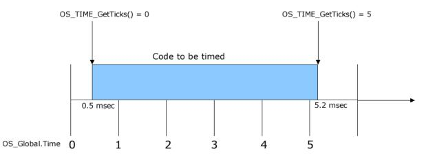
For many applications, low-resolution measurement is sufficient for most of all cases. In those cases, its ease of use as well as its faster computation time are clear benefits when compared to high-resolution measurement. Still, high-resolution measurement may be necessary when highly accurate measurements are mandatory.
